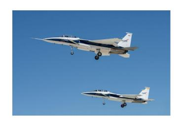
Two of NASA's F-15s are mounted with a state-of-the-art data probe to measure the shock waves of another aircraft flying at supersonic speeds. When the X-59 flies, NASA will use the probe to measure its unique shock waves in flight. Photo credit: Carla Thomas
