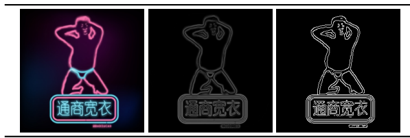
Figure A.7: Two kinds of edge detection. Left, the original image. Center, the image with a Sobel filter applied. Right, the Canny edge detection algorithm.
