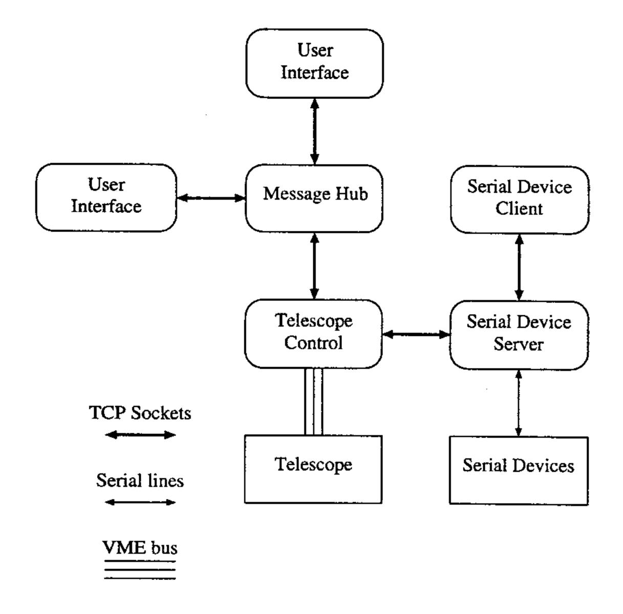
Figure 1: WIYN Control System Architecture
