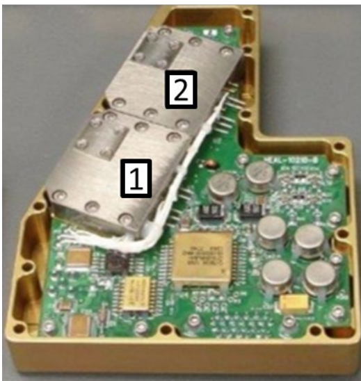
Figure 1. Photograph of a REACH pod with Dos1 and Dos2 labeled. Coordinate axes are also provided, as well as the relationship between incident particle momentum p and the coordinates.
