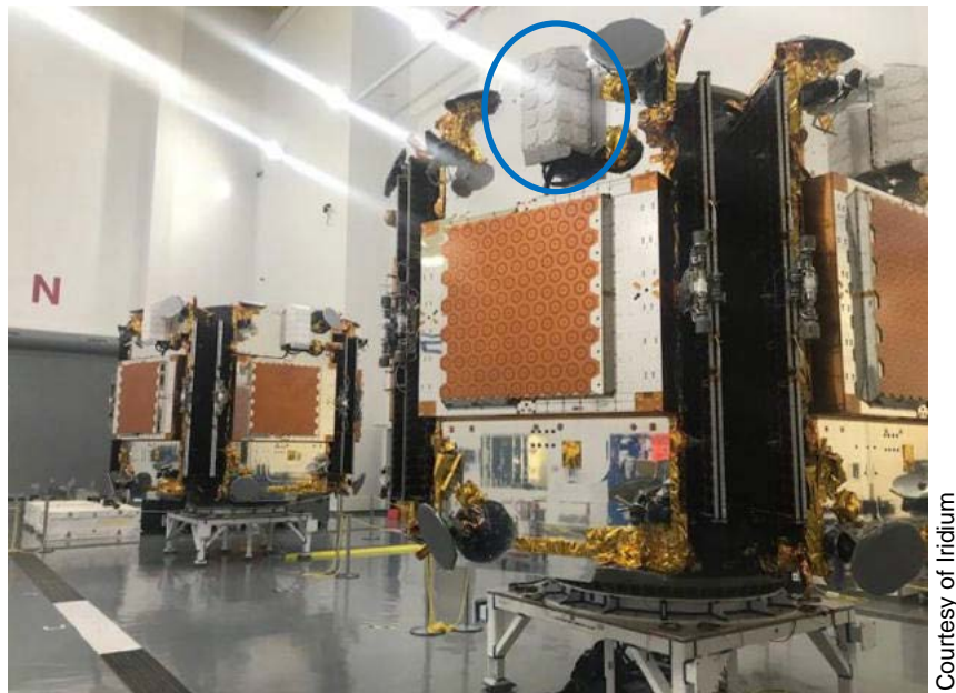
Figure 1. The Iridium satellites prior to launch. The REACH hosted payload is located inside the white hosted payload at the top of the satellite and circled in this figure [1].
